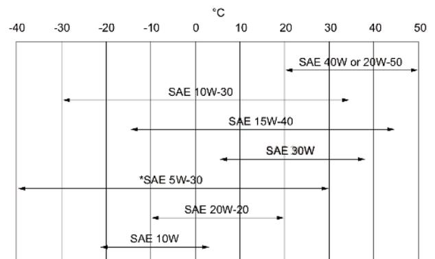
\* Can be used only when available with appropriate diesel rating. For synthetic oil use the recommendation from the oil manufacturer.
